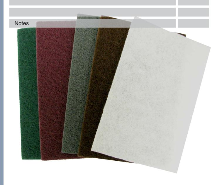
**Hand Pads** are flexible surface finishing abrasive tools mainly used for cleaning, blending, polishing, and finishing a variety of materials. In the manufacturing process non-woven nylon web is impregnated with resins and abrasive grains throughout the web, creating a three-dimensional structure.
