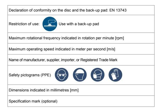
\* EN 13743 marking shows that the producer has followed the essential safety requirements of the European safety standard for fibre discs in order to reduce the risks for the end-user. The markings listed above, except n°6 and 8, are mandatory for products marked EN 13743 on the disc or the packaging.
